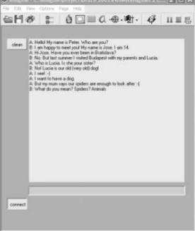
The chat project consists of two buttons, a pane (to display the history of the communication) and an input text box with single line. This text box has a key menu attached: [Enter [net1'mySend]]. There is a net object – named net1 – which is responsible for the entire communication. It consists of two very simple procedures:
